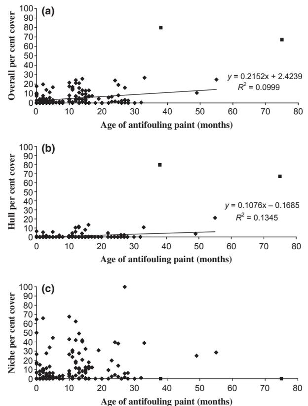
Figure 5 Relationship between age of antifouling paint (months) and (a) overall per cent cover, (b) hull per cent cover and (c) niche per cent cover. Diamonds represent individual boats; squares are statistical outlier points plotted but not part of fit line analyses.
